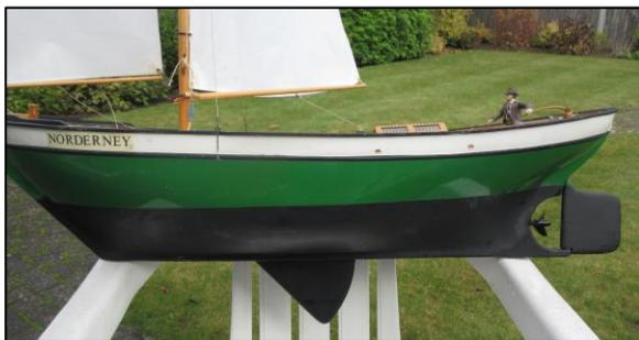
and she sails fine. I think the internal weight has the added effect of making the hull more stable in the water, as there is no 'pendulum' effect with a keel weight lower down.
